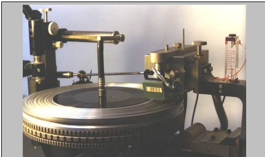
Cutting Lathes, such as the Neumann lathe pictured above, have not changed very much in terms of technology.
